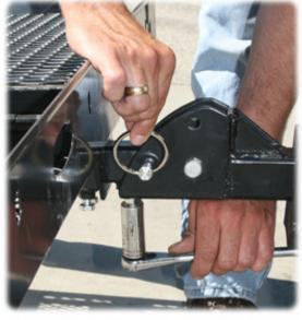
Remove Pin(17) to fold carrier vertical. Replace Pin (17) in top pin hole to secure carrier in the vertical position.
